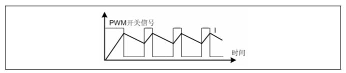
Figure 1-3 Current on load
